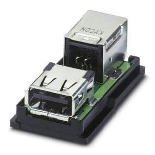
USB socket insert, 4-pos., socket USB type A on socket USB type B, for the Freenet system in the panel mounting frame, IP20 terminal outlet, 19" patch panel and service interface, pluggable from both directions
